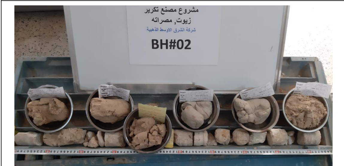
Photo No 10: samples series along depth, BH#02 (Misurata free zone, Misurata city).
