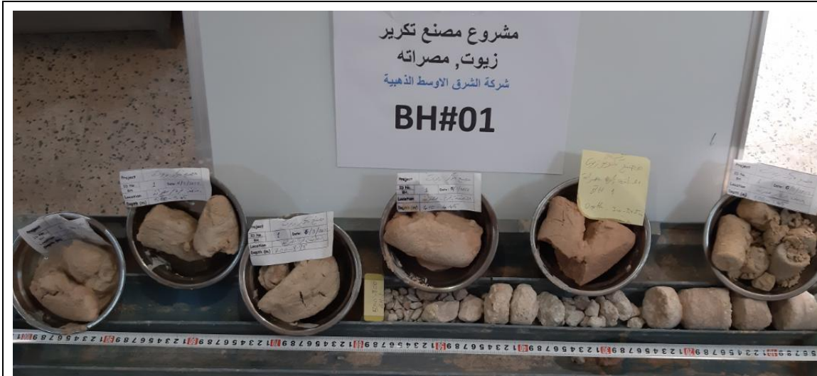
Photo No 9: samples series along depth, BH#01 (Misurata free zone, Misurata city).
