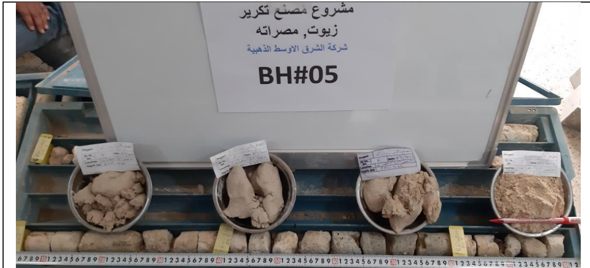
Photo No 13: samples series along depth, BH#05 (Misurata free zone, Misurata city).
