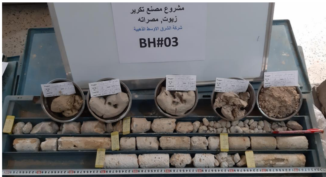
Photo No 11: samples series along depth, BH#03 (Misurata free zone, Misurata city).
